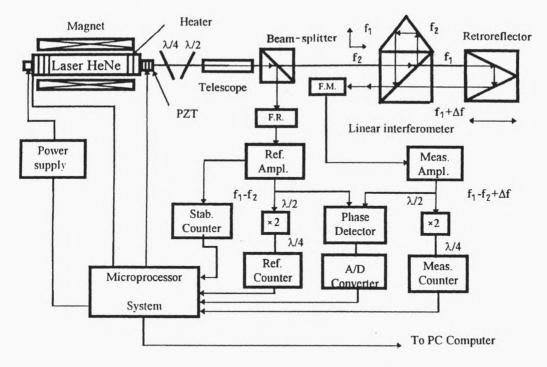
Fig. 2. Block diagram of laser head.  $\lambda/4$  – quarter-wave plate,  $\lambda/2$  – half-wave plate, F.M. – measurement photodetector, F.R. – reference photodetector,  $\times 2$  – multiplier by 2, PZT – piezo-ceramic
