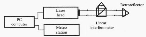
Fig. 1. Block diagram of the laser interferometer LSP-30
