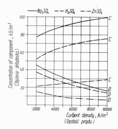
Fig. 5. Concentrate (C) and diluate (D) concentrations versus current density at time T = 30 min.
