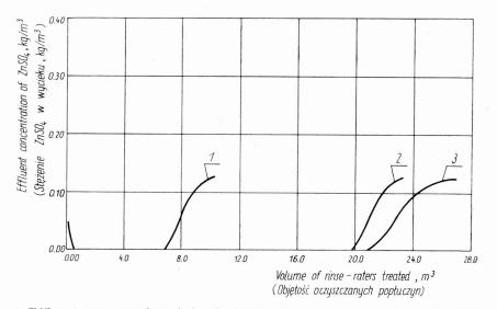
Fig. 1. Effluent concentration of zinc during process of sorption performed on different cation exchangers: 1 - MK-3, 2 - KPS, 3 - X-SD
