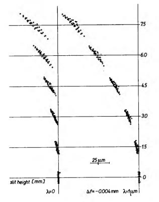
Fig. 7. Spot diagrams for the Littrow system with parabolic mirror
