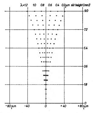
Fig. 10. Curved spectrum lines related to the exit slit. Littrow system. Straight entrance slit, curved exit slit. R-328 mm
