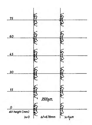
Fig. 4. Spot diagrams for the Czerny-Turner system with spherical mirrors. The vertical scale of the spots are compresse by a factor of 5 to avoid overlapping between neighbourin slit points due to the large astigmatism.  $\Delta f$  is the image plane – Gaussian plane distance
