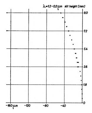
Fig. 11. Spectrum lines with wavelength independent curvature related to the exit slit. Chupp-Grantz system. Curved slits.  $\Phi = 9^{\circ}$ , R = 48.13 mm
