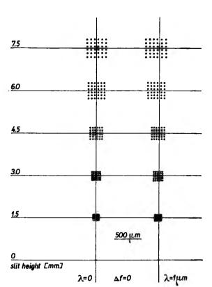
Fig. 5. Spot diagrams for the Czerny-Turner system with parabolic mirrors
