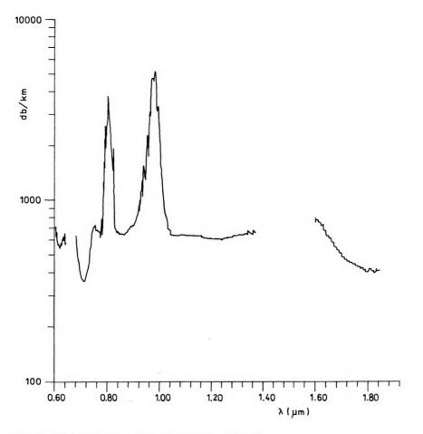
Fig. 2. Attenuation curve for erbium doped silica fiber
