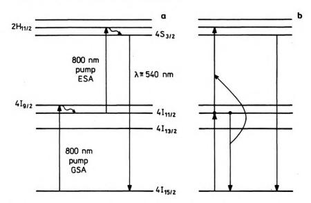
Fig. 3. Simplified energy level diagram of erbium doped silica illustrating infrared-to-visible upconversion. Population of the  ${}^{4}S_{3/2}$  fluorescence level may be caused by excited state absorption (GSA) – **a**, or by an ion pair cooperative process – **b**. Both processes can also be involved simultaneously
