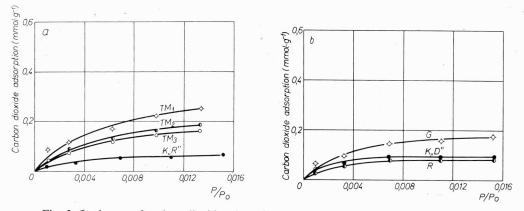
Fig. 3. Isotherms of carbon dioxide adsorption on aluminum coagulation sludge specimens
