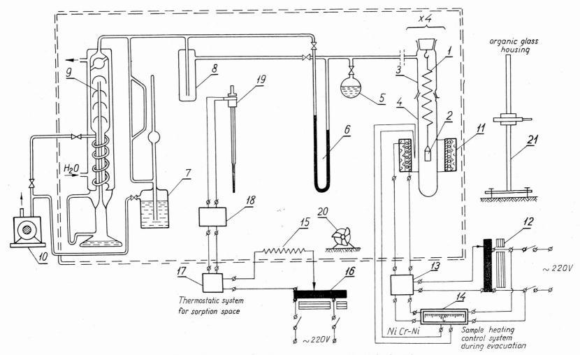
Fig. 2. Scheme of experimental sorption apparatus (description in text) Rys. 2. Schemat doświadczalnej aparatury sorpcyjnej (opis w tekście) a McLeod manometer (7), frezer (8), three-stage diffusion pump (9) to obtain a high vacuum, and oil pump (10) to obtain preliminary vacuum.
