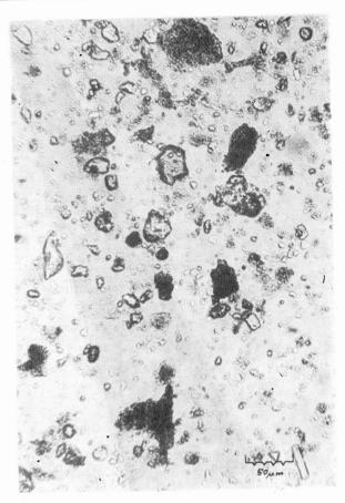
Fig. 1. Microscopic photograph of aluminium coagulation sludge particles from water treatment plant:
