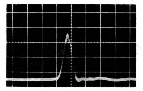
Fig. 8. A pulse of the lasing action of an scintillator excited by a pulse of nitrogen laser. Horizontal scale -5 ns/cm
