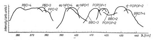
Fig. 4. Selected curves from fig. 3 combined in order to cover the considered spectral range
