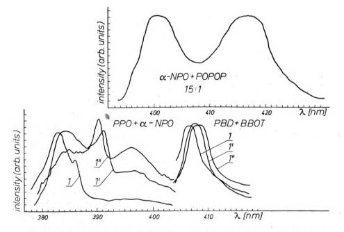
Fig. 5. Curves of laser emission for several three-component mixtures PPO +  $\alpha$ NPO - 1 - 10:1, 1' - 6:1, 1'' 4:1; PBD + BBOT - 1 - 200:1, 1' - 100:1, 1'' - 70:1
