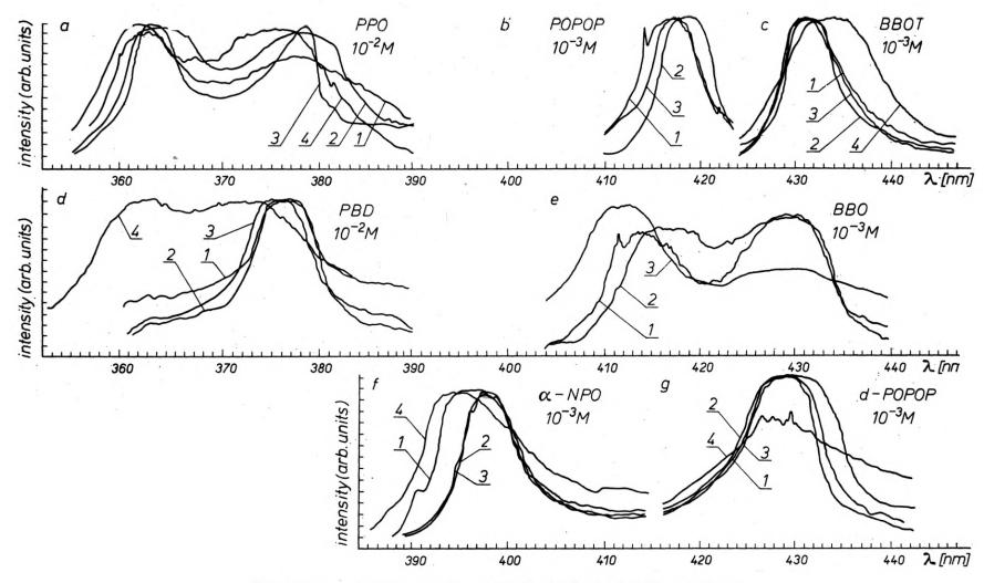
Fig. 3. Laser emission curves for examined scintillators in different solvents
