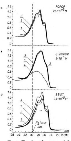
Fig. 1. The absorption curves of the examined organic scintillators in four solvents: 1) toluene, 2) o-xylene, 3) p-xylene, 4) ethanol. The position of the nitrogen laser emissive line is marked
