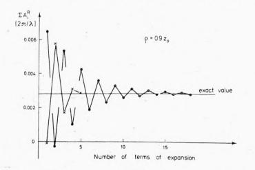
Fig. 2. Spherical aberration in the vicinity of ρ = 1 − an illustration of the increase of convergence of relations (3) and (8)
