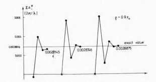
Fig. 3. Spherical aberration of the  $\Phi_R$  for  $z_c = 1.2 z_o$  and  $z_r = 1.1 z_o$  computed from the relation (8) by taking into account of the four, five and six terms of the expansion
