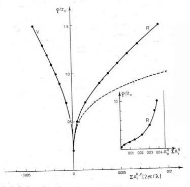
Fig. 1. Spherical aberration of wavefront  $\Phi_R$  and  $\Phi_V$  for  $z_c = 1.2 z_0$ ,  $z_r = 1.1 z_0$ ; •---• total spherical aberration,  $\times - - \times$  spherical aberration of third order of  $\Phi_R$
