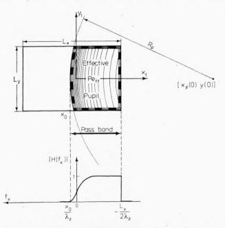
Fig. 3. Analogy between isoplanatic HOS and band-pass filter; transfer function H is shown for  $f_{II} = 0$
