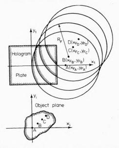
Fig. 2. Illustration of OTF influence, as a masking operation, for discrete point of the object
