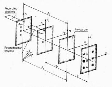
Fig. 4. Geometry of generalized Vander-Lugt filter
