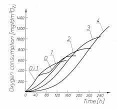
oxygen consumption have been stated. These differences were found in the remaining samples in which the percent of wastewaters from wet dedusting was higher. Lower oxygen consumptions in the samples were due to the toxicity of industrial wastewater pollutants for non-adapted microorganisms. The toxic effect enhanced by the increasing percentage of industrial wastewater in the mixture treated, was reflected in smaller amounts of the oxygen consumed.
