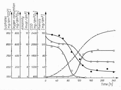
Fig. 3. Biological treatment of wastewater from wet dedusting. Dilution with municipal wastewater 1:3
