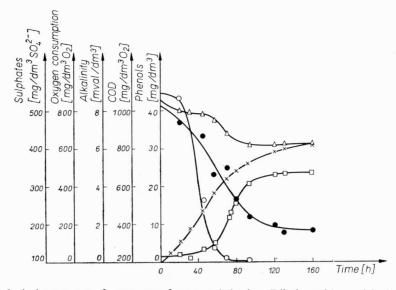
Fig. 2. Biological treatment of wastewater from wet dedusting. Dilution with municipal wastes 1:9 △ - alkalinity, x - oxygen consumption, • - COD, □ - sulphates
