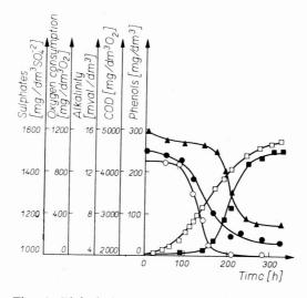
Fig. 4. Biological treatment of wastewater from wet dedusting. Dilution with municipal wastewater 1:1
