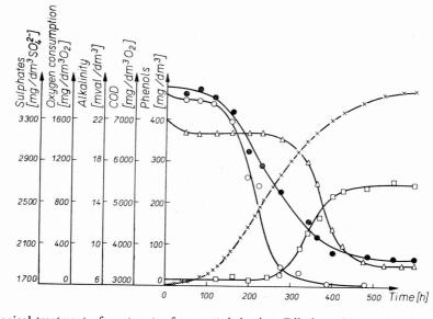
Fig. 5. Biological treatment of wastewater from wet dedusting. Dilution with municipal wastewater 9:1
