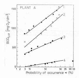
Fig. 3. Statistical correlation of raw wastes and effluents from various unit processes *1* - raw BOD<sub>5</sub>, 2 - screened, 3 - after chemical precipitation 4 - after activated sludge
