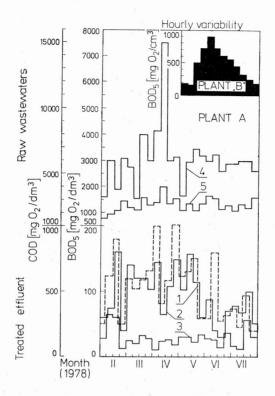
Fig. 2. Variability of COD and BOD in raw and treated effluent from plant A Treated wastes:  $1 - \text{COD}_{nf}$ ,  $2 - \text{BOD}_{5,nf}$ ,  $3 - \text{BOD}_{5f}$ Raw wastes:  $4 - \text{COD}_{nf}$ , BOD<sub>5,nf</sub>
