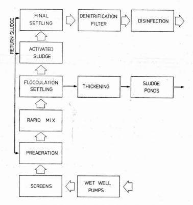
Fig. 4. Layout of a typical plant – farm ARys. 4. Schemat typowej oczyszczalni – ferma A
