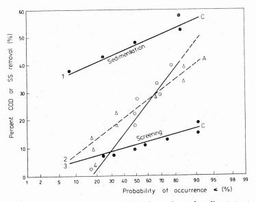
Fig. 5. Efficiency of screening at plant A and C and experimental settling tests at plant C: 1 - COD removal at plant C - settling, 2 - SS removal (A) - screening, 3, 4 - COD removal (plant A and C, respectively) - screening
