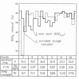
Fig. 13. BOD removal in activated sludge (line 1) and for the whole plant (line 2) plant A:  $1 - BOD_{s,f}$ ,  $2 - BOD_{s,nf}$
