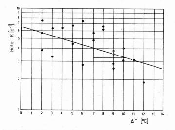
Fig. 10. Determination of the temperature correction factor for piggery wastes – plant A
