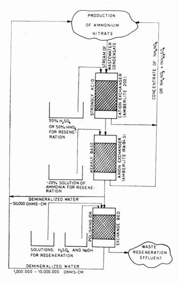
Fig. 4. Recycling of ammonia, nitrates and water from wastewater of ammonium nitrate processing to technological process by ion exchange method
