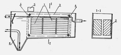
Fig. 2. Multi-tier settlers operating in transversal mode
