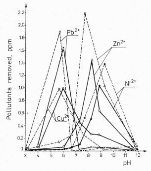
Fig. 4. Effect of pH on the increment of heavy metals removal in alum (-----90 ppm) or ferric sulfate (----90 ppm) coagulation and 2-hour sedimentation
