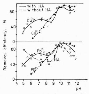
Fig. 3. Effect of pH value and humic acids on lead and copper removal in the following processes: pH adjustment and filtration through a filter paper
