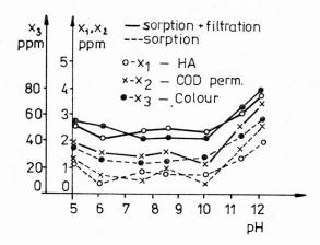
Fig. 2. Relationship between pH of aqueous solutions and sorption efficiency on pulverized activated carbon Carbopol Z-4
