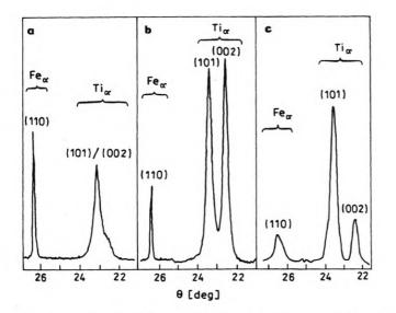
Diffractograms of titanium layers deposited on the carbon steel substrate using the dc magnetron sputtering method immediately after deposition (a), conventional annealing at a temperature of 400° C (b) and after irradiating with a CO<sub>2</sub> laser of power density  $Q \simeq 26 \times 10^7$  W/m<sup>2</sup> and speed of beam sweeping v = 0.27 m/s (c). Radiation CoK<sub>co</sub> continuous recording
