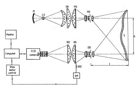
Fig. 1. Schematic representation of the projection moire system. LS – light source, M – mirror, CN – condenser, PG – projection grating, PO – projection objective, OB – object under test, DO – detection objective, DG – detection grating, RO – relay optics, SM – system motor, DSC – driving screw control
