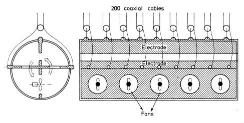
Fig. 1. Laser tube construction: a - transversal cross-section, b - longitudinal cross-section of the laser tube
