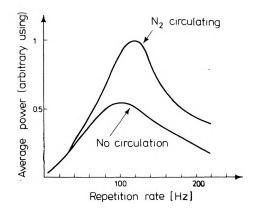
Fig. 2. Average output power vs. repetition rate
