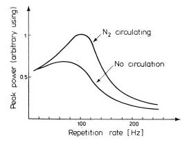
Fig. 3. Peak power vs. repetition rate. Arbitraty unit equals circa 300 kW. Output power was not too high because of relatively high wave resistance of charging cables
