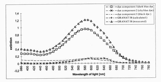
Fig. 2. The spectrum of dyeing bath components of dyeing bath GRANAT 58
