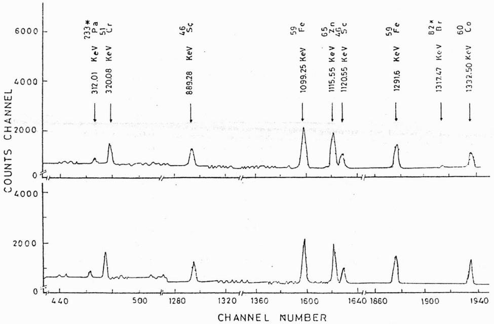
Fig. 2. Portion spectra of shoot and root of water hyacinth for site A (El-Mahsama drain)
