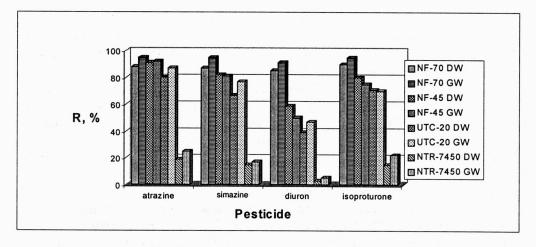
Fig. 1. The efficiency of pesticide removal by nanofiltration (R - rejection, DW - distilled water, GW - ground water) [22]
