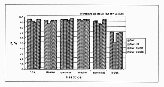
Fig. 2. The influence of humic acids (HA) and inorganic acids on pesticide removal by nanonofiltration (R - rejection, DW - distilled water)
