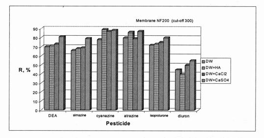
Fig. 3. The influence of humic acids (HA) and inorganic acids on pesticide removal by nanonofiltration (R - rejection, DW - distilled water)
