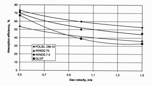
Fig. 1. Absorption efficiency as a function of gas velocity in empty column;  $L = 10 \text{ m}^3/\text{m}^2\text{h}$ ,  $C_{g1} = 400 \text{ mg/m}^3$ ,  $T_l = T_g = 293 \text{ K}$ ,  $C_c = 0 \text{ g/m}^3$
