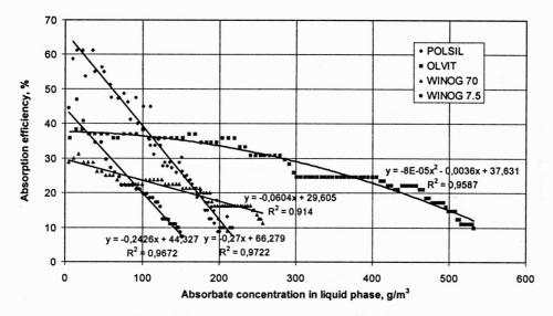
Fig. 2. Absorption efficiency as a function of trichloroethylene concentration in liquid phase;  $C_{g1} = 400 \text{ mg/m}^3$ ,  $L = 10 \text{ m}^3/\text{m}^2$ h, v = 1 m/s,  $T_l = T_g = 293 \text{ K}$
