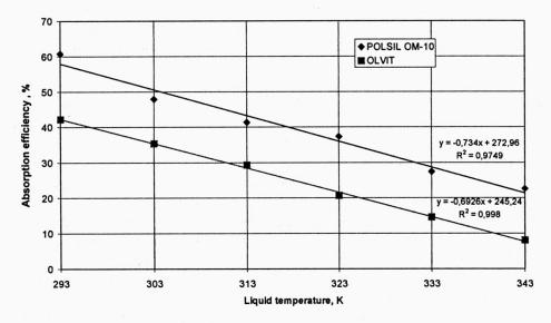
Fig. 4. Absorption efficiency as a function of temperature;  $L = 10 \text{ m}^3/\text{m}^2\text{h}$ ,  $C_{g1} = 400 \text{ mg/m}^3$ , v = 1 m/s,  $T_g = 293 \text{ K}$ ,  $C_c = 0 \text{ g/m}^3$
