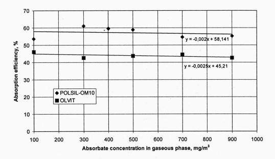
Fig. 3. Absorption efficiency as a function of trichloroethylene concentration in gaseous phase;  $L = 10 \text{ m}^3/\text{m}^2\text{h}$ , v = 1 m/s,  $T_l = T_g = 293 \text{ K}$ ,  $C_c = 0 \text{ g/m}^3$
