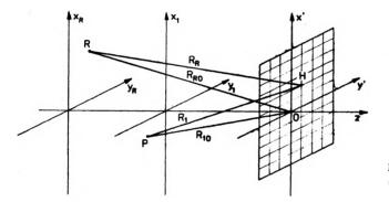
Fig. 1. Geometry of hologram recording
