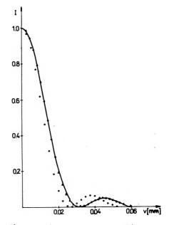
Fig. 4. Light intensity distribution in the image calculated for different numbers of rays taken into account hologram No. 1 (0000 -  $\Delta y = 0.48$ , N = 5; -----  $\Delta y = 0.00375$ , N = 534;  $\Delta \Delta x = 0.06$ , N = 34)
