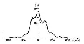
Fig. 7. Light intensity distribution in the image calculated for different numbers of rays taken into account = hologram No. 2. (-. -  $\Delta y = 0.25$ , N = 17;,  $-\Delta y = 0.05$ , N = 81; - -  $\Delta y = 0.0005$ , N = 1601)
