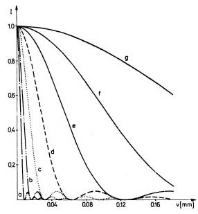
In the following test the effect of hologram size inoreasing at the constant density of rays has been investigated. The image analysed being aberration free, the light intensity distribution in this image should depend only on the diffraction of the hologram
