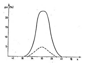
Fig. 2. Absorption band of a glass: solid line - the sample irradiated with X-rays, dotted line - th sample exposed to UV radiation
