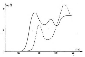
Fig. 4. TSEE curve of a glass irradiated with ultraviolet N<sub>2</sub> laser
