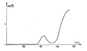
Fig. 3. TSEE curve from nonirradiated glass sample
