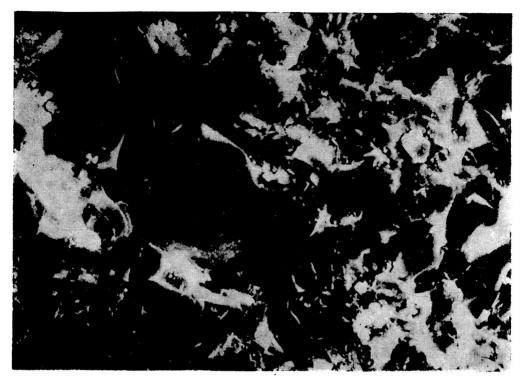
Fig. 6. Scanning electron micrograph of heated glass sample irradiated with  $N_s$  laser
