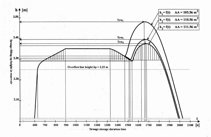
Fig. 3. Effect of storage chamber surface level on the position of sewerage in a complete storage phase in the two-chamber reservoir of the CONTRACT type
