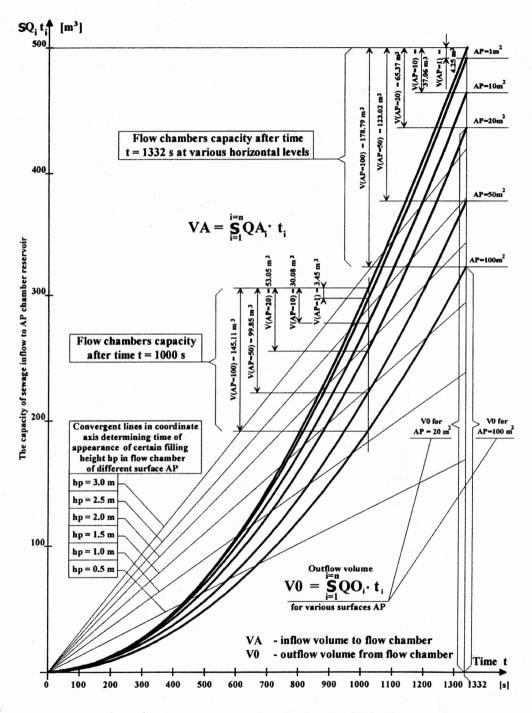
Fig. 1. Diagrams of sewage storage in flow chamber of multi-chamber reservoirs
