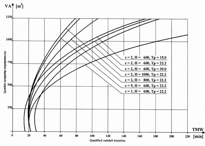
Fig. 6. Effect of model parameters *c*, *H* and *Tp* on retention capacity area of two-chamber reservoirs and qualified rainfall
