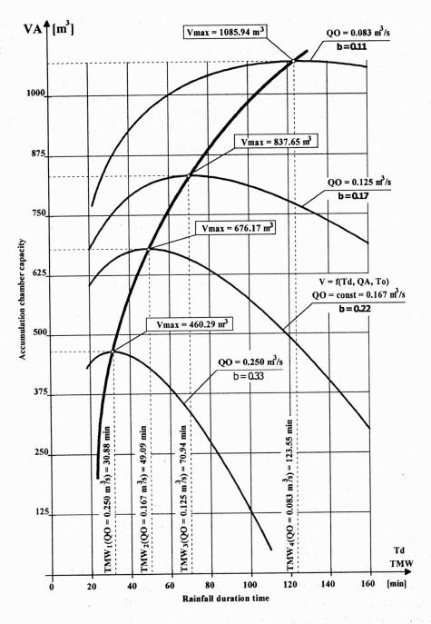
Fig. 5. An example of the result of sewage storage simulation in two-chamber reservoir of the CONTRACT type
