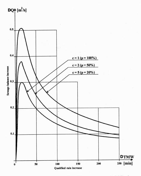
Fig. 4. Diagram of sewage balance for variable qualified time and assumed reliability degree of two-chamber storage reservoir operation
