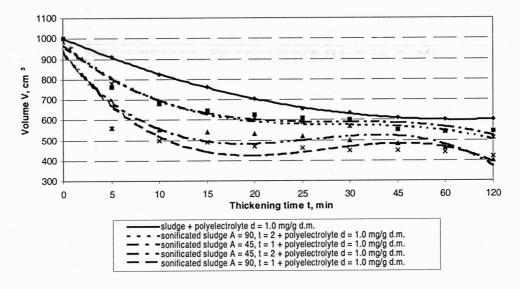
Fig. 2. The process of gravitational thickening of sludge prepared with polyelectrolyte only and ultrasounds + polyelectrolyte
