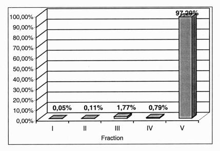
Fig. 2. Contributions of particular fractions to the total content of aluminium, mean values from all the samples studied
