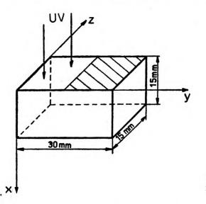
Fig. 1. Orientation of sample during irradiation
