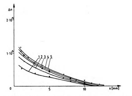
Fig. 4. Dependence of the changes of refractive index on the penetration depth of UV radiation for different temperatures at which the sample was kept during irradiation: 1 - 25 °C 2 - 50 °C, 3 - 100 °C, 4 - 160 °C, 5 - 210 °C. Exposure time - 1 h, the illuminating 400 Watt lamp was used
