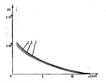
Fig. 2. Dependence of the changes of refractive index on the penetration depth of UV radiation for different exposure times: 1 - 20 min., 2 - 40 min., 3 - 60 min. During the irradiation the sample was kept at the 300 °C, the 400 Watt illuminating lamp was used
