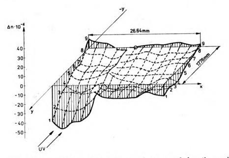
Fig. 8. Changes of refractive index in the x, y plane averaged along the sample thickness in the z-axis direction. Viewing direction perpendicular to that of irradiation. The numbers denote the successive scanning lines
