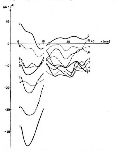
Fig. 7. Change of refractive index averaged along the total sample thickness for the successive scanning lines. The viewing direction perpendicular to that of irradiation
