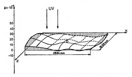
Fig. 10. Changes of refraction index in the direction of irradiation
