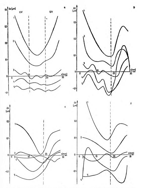
Fig. 9. Changes of the linear sizes of the glass sample after irradiation and application of the steady electric field. The numbers denote the successive scanning lines:  $\mathbf{a}$  – after irradiation without the applied field,  $\mathbf{b}$  – after application of the +12 kV voltage during 1 h,  $\mathbf{c}$  – after application of the -12 kV voltage during 1 h,  $\mathbf{d}$  – permanent changes
