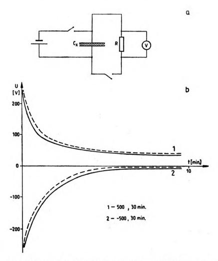
Fig. 2. Determination of the relaxation curves:  $\mathbf{a}$  — measuring set-up,  $\mathbf{b}$  — relaxation curves describing the irradiated (continuous line) and nonirradiated (broken line) parts ( $C_x$  — investigated sample, R — resistor, V — voltmeter)
