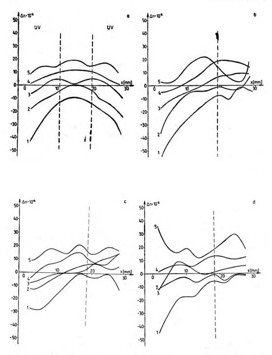
Fig. 8. Changes of refractive index in the glass sample after its irradiation and application of the steady electric field. The numbers denote the successive scanning lines:  $\mathbf{a}$  — after irradiation without applied field,  $\mathbf{b}$  — after application of the +12 kV voltage during 1 h,  $\mathbf{c}$  — after application of the -12 kV voltage during 1 h,  $\mathbf{d}$  — permanent change
