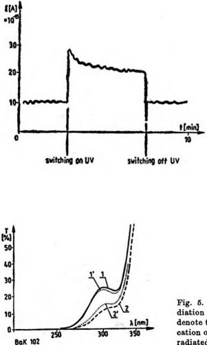
Fig. 4. Current flow observed in the glass sample during the irradiation by UV radiation
