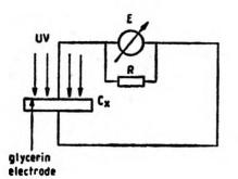
Fig. 3. Measuring setup for current flow  $(O_x - investigated sample, E - electrometer, R - resistor)$
