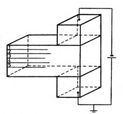
Fig. 7. Sample orientation at the presence of the external electric field (1-5 - scanning) lines)
