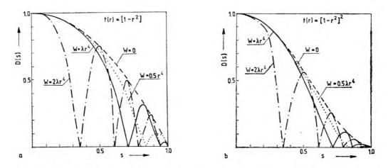
Fig. 7. Contrast change D(s) for amplitude test in the optical system with aberrations  $W(r) = 0.5\lambda r^4$ ,  $\lambda r^4$ ,  $2\lambda r^4$  apodized with the functions:  $t(r) = 1 - r^2$ , m = 0 (a),  $t(r) = (1 - r^2)^2$ , m = 0 (b)
