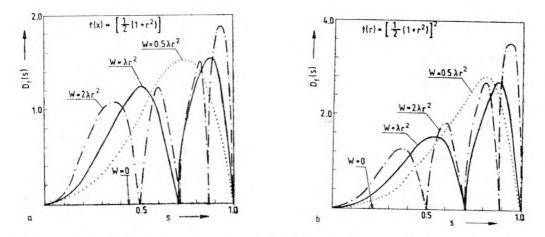
Fig. 10. Contrast change D(s) for phase test in the optical system with aberrations  $W(r) = 0.5\lambda r^2$ ,  $\lambda r^2$ ,  $2\lambda r^2$  apodized with the functions:  $t(r) = 1/2(1+r^2)$ , m = 0 (a),  $t(r) = [1/2(1+r^2)]^2$ , m = 0 (b)
