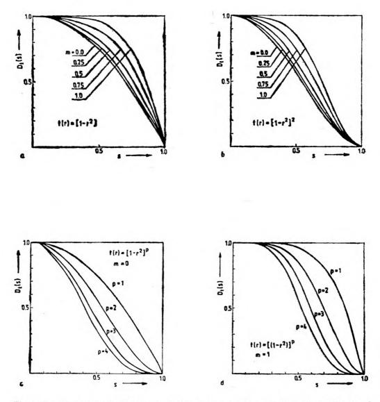
Fig. 2. The effect of apodization t(r) on the image contrast of amplitude test for:  $t(r) = 1 - r^2$ (a),  $t(r) = (1 - r^2)^2$  (b),  $t(r) = (1 - r^2)^p$ , p = 1, 2, 3, 4; m = 0 (c),  $t(r) = (1 - r^2)^p$ , p = 1, 2, 3, 4; m = 1 (d)
