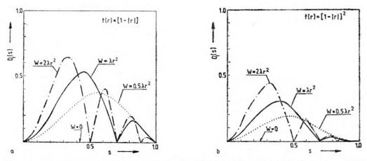
Fig. 14. Contrast change D(s) for phase test in the optical system with aberrations  $W(r) = 0.5\lambda r^2$ ,  $\lambda r^2$ ,  $2\lambda r^2$  apodized with the functions: t(r) = 1 - |r|, m = 0 (a),  $t(r) = (1 - |r|)^2$ , m = 0 (b)
