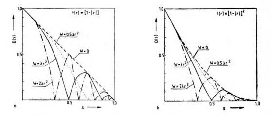
Fig. 8. Contrast change D(s) for amplitude test in the optical system with aberrations  $W(r) = 0.5\lambda r^2$ ,  $\lambda r^2$ ,  $2\lambda r^2$  apodized with the functions: t(r) = 1 - |r|, m = 0 (a),  $t(r) = (1 - |r|)^2$ , m = 0 (b)
