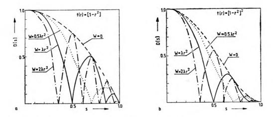
Fig. 6. Contrast change D(s) for amplitude test in the optical system with aberrations  $W(r) = 0.5 \lambda r^2$ ,  $\lambda r^2$ ,  $2\lambda r^2$  apodized with the functions:  $t(r) = 1 - r^2$ , m = 0 (a),  $t(r) = (1 - r^2)^2$ , m = 0 (b)
