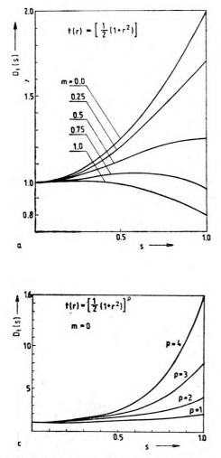
Fig. 1. The effect of amplitude apodization t(r) on the image contrast of amplitude test for:  $t(r) = 1/2(1+r^2)$ (a),  $t(r) = [1/2(1+r^2)]^2$  (b), t(r) $= [1/2(1+r^2)]^p$ , p = 1, 2, 3, 4; m = 0 (c),  $t(r) = [1/2(1+r^2)]^p$ , p = 1, 2, 3, 4; m = 1 (d)
