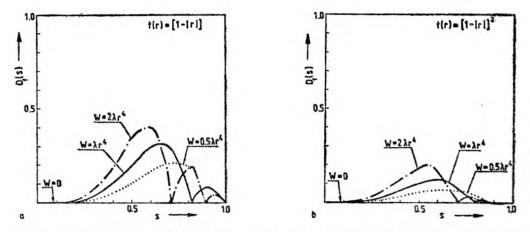
Fig. 15. Contrast change  $D^{l}(s)$  for phase test in the optical system with aberrations  $W(r) = 0.5\lambda r^{4}$ ,  $\lambda r^{4}$ ,  $2\lambda r^{4}$  apodized with the functions: t(r) = 1 - |r|, m = 0 (a),  $t(r) = (1 - |r|)^{2}$ , m = 0 (b)
