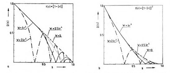
Fig. 9. Contrast change D(s) for amplitude test in the optical system with aberrations  $\overline{W}(r) = 0.5\lambda r^4$ ,  $\lambda r^4$ ,  $2\lambda r^4$  apodized with the functions: t(r) = 1 - |r|, m = 0 (a),  $t(r) = (1 - |r|)^3$ , m = 0 (b)
