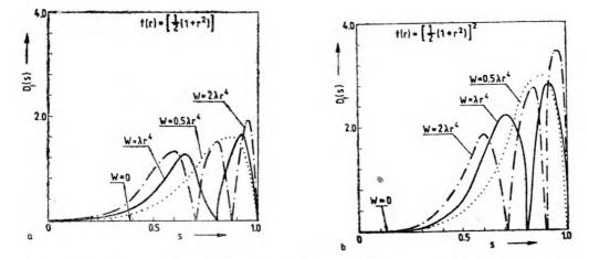
Fig. 11. Contrast change D(s) for phase test in the optical system with aberrations  $\overline{W}(r) = 0.5\lambda r^4$ ,  $\lambda r^4$ ,  $2\lambda r^4$  apodized with the functions  $t(r) = 1/2(1+r^2)$ , m = 0 (a),  $t(r) = [1/2(1+r^2)]^2$ , m = 0 (b)
