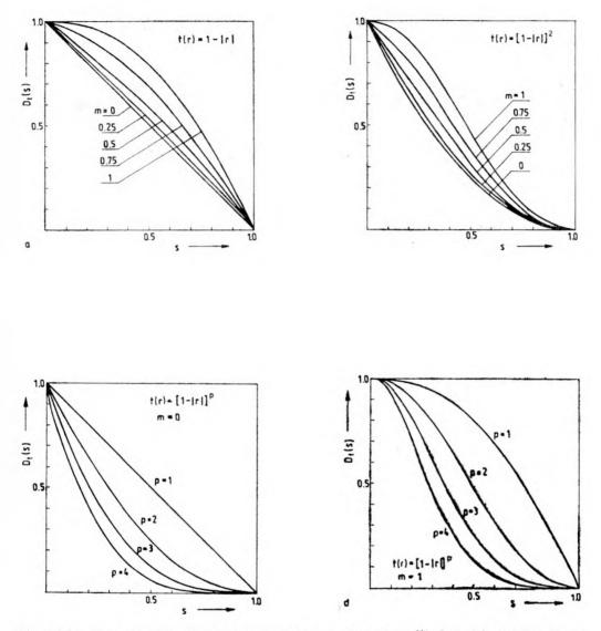
Fig. 3. The effect of apodization t(r) on the image contrast of amplitude test for: t(r) = 1 - |r|(a),  $t(r) = (1 - |r|)^2$  (b),  $t(r) = (1 - |r|)^p$ , p = 1, 2, 3, 4: m = 0 (c),  $t(r) = (1 - |r|)^p$ , p = 1, 2, 3, 4: m = 1 (d)
