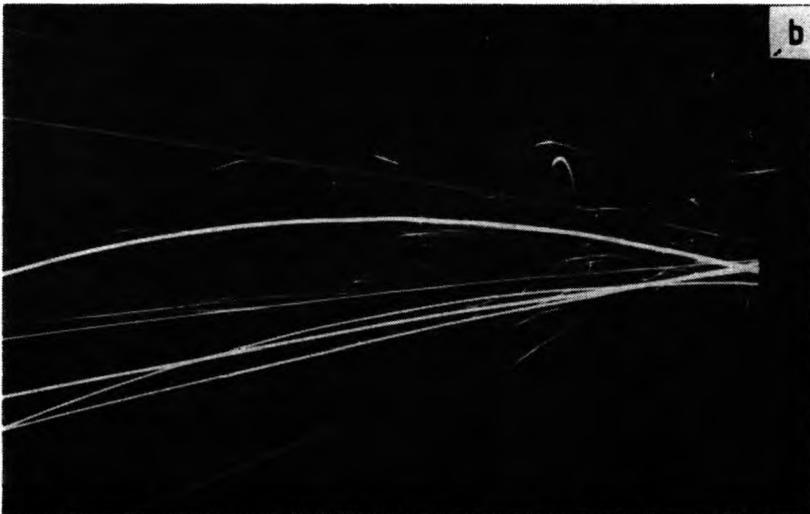
Fig. 33. Pictures of a long exposure time photography of electrodes erosion process in electrode configuration used in medium-voltage disconnector for two SAP current: a -  $I = 800$  A, b -  $I = 2400$  A
