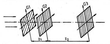
Fig. 1. Geometry of the double-grating diffraction system. G1 and G2 – linear rulings form ming the double-diffraction configuration, G3 – linear ruling for detecting the Fresne field behind the grating G2
