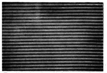
Fig. 2. Moiré fringes observed in the plane of the detection grating G3 due to the beat phenomenon between the self-image of G2 and grating G3
