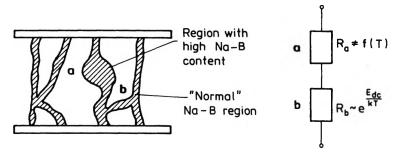
Fig. 5. Schematic diagram of the leakage filament
