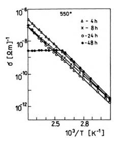
Fig. 3. Dependence of dc conductivity on temperature for the glasses before and after heat treatment at  $550^{\circ}$ C
