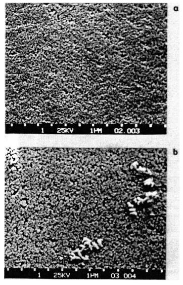
Fig. 4. EM micrographs of investigated glasses (a - heat treatment at 550°C for 4 h, b - heat treatment at 570°C for 48 h)
