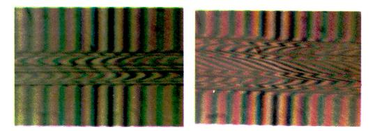
Fig. 3. Splitting of the pattern of a four-layer optical fibre, 4wHB [3], in the fringe interference field:  $\mathbf{a}$  - objective magnification 10×, photograph magnification 130×,  $\mathbf{b}$  - objective magnification 20×, photograph magnification 260× ( $n_m = n_p = 1.5083$ ,  $t = 17.5^{\circ}$ C)
