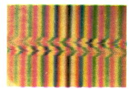
Fig. 1. Complete splitting of the pattern of a twolayer optical fibre, 2wBc, in the striated interference field:  $n_m = n_p = 1.5373$ . Photograph magnification  $130 \times$ ,  $t = 19.7^{\circ}$  C
