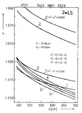
Fig. 5. Dispersion curves of fibre, 2wLS (1 - cladding, 2 - core), immersion fluids (curves 3, 4, 5 and 6) and initial glass used for the cladding and core (curves 1' and 2')
