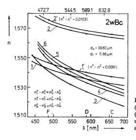
Fig. 4. Dispersion curves of fibre, 2 wBe(1 - cladding, 2 - core), immersion fluids (curves 3, 4, 5 and 6) and the initial glass used for the cladding and core (curves 1' and 2')
