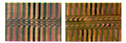
Fig. 2. Splitting of the pattern of a high-aperture optical fibre, 2wLS, in the fringe interference field: **a** – objective magnification  $10 \times$ , photograph magnification  $130 \times$ , **b** – objective magnification  $40 \times (n_m = n_p = 1.5682, t = 17.5^{\circ} \text{C})$
