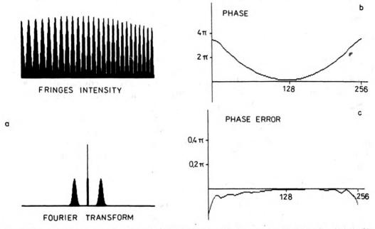
Fig. 1. Fringe pattern cross-section given by 256 intensity samples: its spectrum (a), the retrieved phase (b) and the distribution of the phase errors (c)
