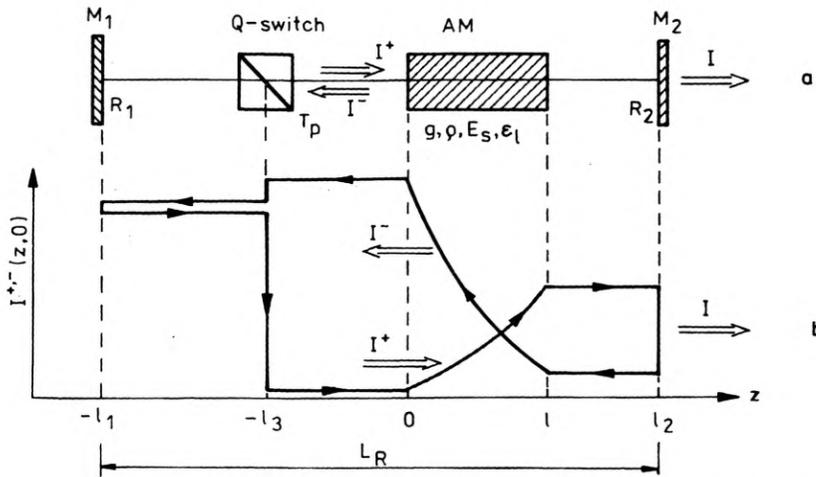
Fig. 1. Scheme of the laser system:  $M_1, M_2$  – mirrors, AM – active medium (a), and initial photon flux distribution  $I^+, I^-$  inside the resonator (b)
