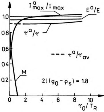
Fig. 4. Influence of Q-switching-off time on the differences of output pulse parameters determined on the basis of SM and AM for  $2l(g_0 - \rho_s) = 1.8$  (where parameter with index "a" denotes the value determined on the basis of the AM model)
