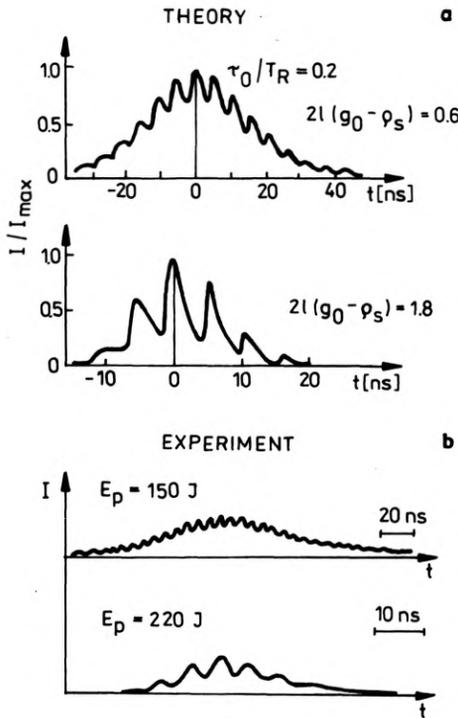
Fig. 3. Shapes of output pulses for different amplifications  $2l(g_0 - \rho_s)$  - a, and exciting energies  $E_p$  - b. The shown oscillograms have been obtained on a classical YAG:Nd<sup>3+</sup> laser system containing electro-optic Q-switch composed of Pockels cell and polarizer
