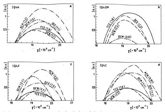
Lasing spectra of investigated dyes in selected solvents (in brackets optimal concentrations [mol/l] are given)
