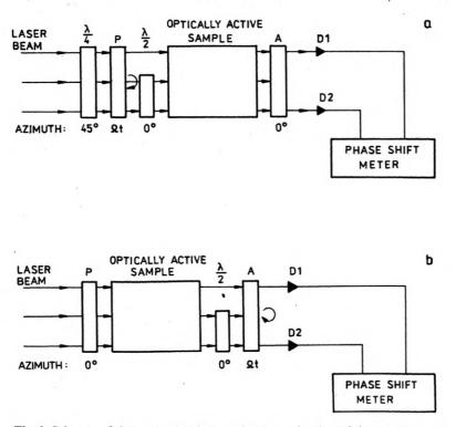
Fig. 2. Schemes of the measuring systems for determination of the rotation angle of polarization azimuth with the use of the technique of phase modulation with a half-shadow element.  $\mathbf{a}$  - rotating polarizer as the modulating element,  $\mathbf{b}$  - rotating analyser as the modulating element
