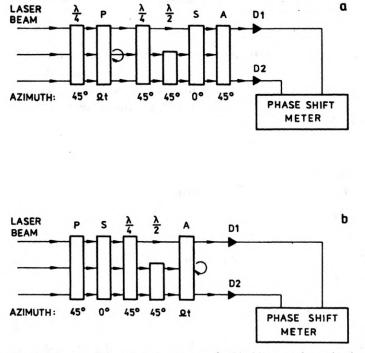
Fig. 1. Schemes of the measuring systems for birefringence determination with the use of the technique of the phase modulation with application of the half-shadow element.  $\mathbf{a}$  – configuration of the Senarmonte inverse compensator,  $\mathbf{b}$  – configuration of the Senarmonte direct compensator
