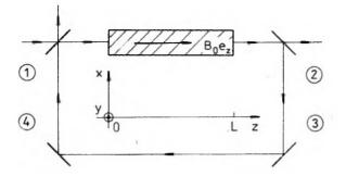
Fig. 1. Nonlinear ring resonator (1-4 mirrors)
