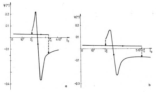
Fig. 4. Bistability of the orientation angle of the polarization ellipse referring to the phase increases:  $\Phi_{\perp} = \Phi_{\parallel} = \pi/6$  (a),  $\Phi_{\perp} = \pi/3$ ,  $\Phi_{\parallel} = \pi/2$  (b)
