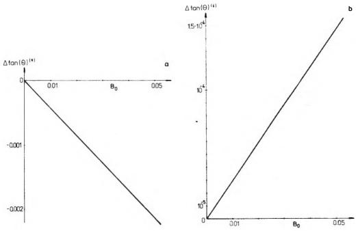
Fig. 7. Heights of the nonlinear "jumps" of the ratio of the polarization ellipse semiaxes of the transmitted light as functions of the external magnetic field referring to the incident light intensities:  $\mathbf{a} - I_0 = I_0^{\dagger}$ ,  $\mathbf{b} - I_0 = I_0^{\dagger}$
