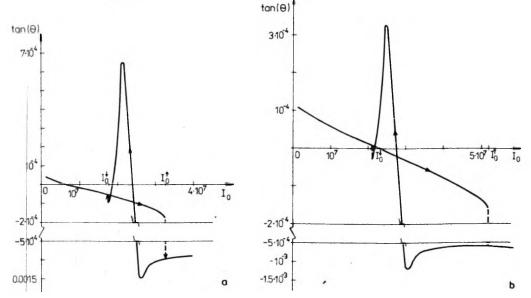
Fig. 3. Bistability of the ratio of the polarization ellipse semiaxes referring to the phase increases:  $\Phi_{\perp} = \Phi_{\parallel} = \pi/6$  (a),  $\Phi_{\perp} = \pi/3$ ,  $\Phi_{\parallel} = \pi/2$  (b)
