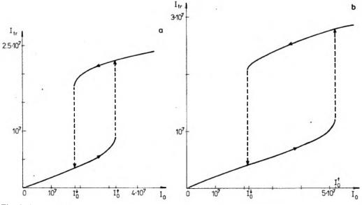
Fig. 2. Intensity bistability in the ring resonator referring to the phase increases:  $\Phi_{\perp} = \Phi_{\parallel} = \pi/6$ (a), and  $\Phi_{\perp} = \pi/3$ ,  $\Phi_{\parallel} = \pi/2$  (b)
