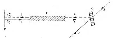
Fig. 1. Experimental arrangement: 1-input beam carrying picture information, 2-reference beam, 3-reading beam, 4-phase conjugate beam retraversing the fiber (F-fiber, K-element generating a phase conjugate signal, P-observation plane of the input signal  $S_0$  and the recovered conjugated signal  $S_0^*$ )
