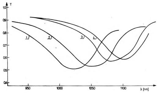
Fig. 2. Spectral lines of selective transmission of the mixture V for temperatures: 1 - 19.7, 2 - 22.5, 3 - 25.1, 4 - 26.6 °C (T - relative transmission)
