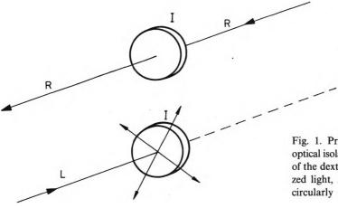
Fig. 1. Principle of operation of the optical isolator: I – isolator, R – beam of the dextrorotatory circularly polarized light, L – beam of leavorotatory circularly polarized light
