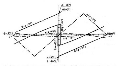
Fig. 6. Changes of ellipticity  $\varepsilon$  (-----) and azimuth  $\theta$  (-·-) as a function of angle position of second loop  $\Phi$ . As a parameter the angle position of first loop  $\varphi$  was used
