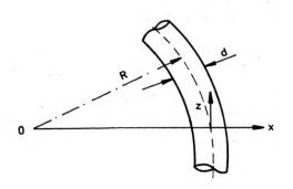
Fig. 2. Bend of the optical fiber with the curvature radius R
