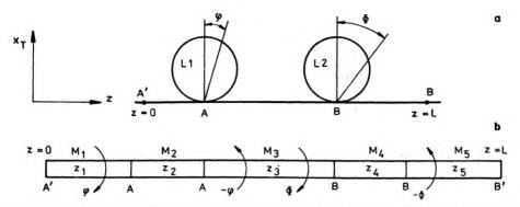
Fig. 4. Matrix description of the loops L1 and L2: the accepted system of coordinates (a) and the matrix representation of PT (b)
