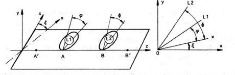
Fig. 3. Polarization transformer and the accepted system of coordinates,  $\xi$  – angle between the laboratory system (x, y) and plane of the loop rolling and mounting,  $\varphi$  – angle of the turn of the loop L1,  $\phi$  – angle of the turn of the loop L2
