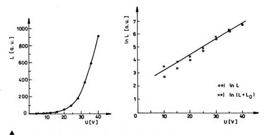
Fig. 4. Voltage dependence of the intensity of electroluminescence of the cadmium electrode after 12 min anodic oxidation at constant voltage of 40 V
