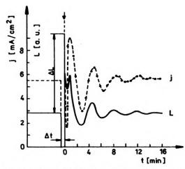
Fig. 6. Anode flash  $\Delta L$  and oscillations of the intensity L of electroluminescence and the current density j in the system switched on after 30 s time lapse. Before switching off the cadmium electrode was formed at a constant voltage of 40 V
