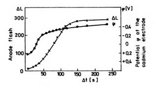
Fig. 7. Anode flash  $\Delta L$  and the potential  $\varphi$  of the cadmium electrode versus the duration of the time lapse  $\Delta t$  between switching off the electrolytic cell and switching it on again
