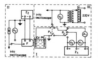
Fig. 1. Scheme of the apparatus for measurements of the electroluminescence accompanying the anodic oxidation of metals:  $Z_1$  – battery,  $Z_2$ – high-voltage supply ZWN-2.5. F – photomultiplier FEU-38
