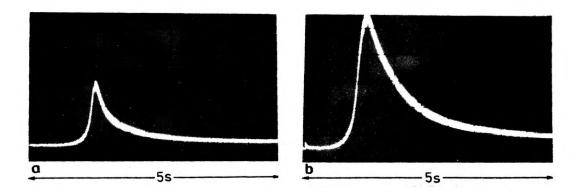
Fig. 3. Oscilloscope traces of the change in the electroluminescence intensity during the early stage of anodic oxidation of cadmium at a constant voltage of 40 V:  $\mathbf{a}$  – Cd plate directly after the chemical cleaning,  $\mathbf{b}$  – Cd plate chemically cleaned and then oxidized by 1 h tempering at 300° C in air under atmospheric pressure
