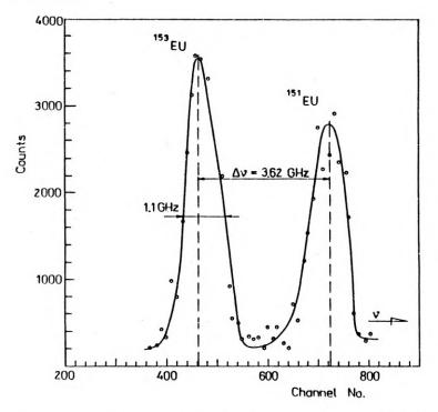
Fig. 2. Optical spectrum of natural Eu mixture, at a laser wavelength  $\lambda = 576.5$  nm
