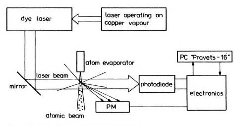
Fig. 1. Functional diagram of the laser spectroscopy
