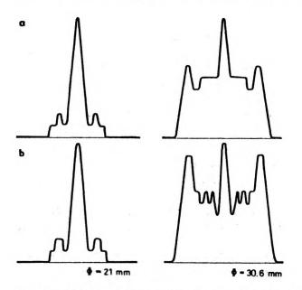
Fig. 4. Normalized near-field laser intensity distributions for small signal gain for curve 1 (a) and 3 (b) of Fig. 1 at two values of diaphragm diameter  $\Phi$ . The central intensity on the resonator axis is used for normalization
