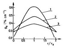
Fig. 1. Gaussian small signal gain variations along the gas flow directions [3] obtained by fitting experimental data corresponding to partial pressures  $p(CO_2)/p(N_2)$  equal to 1/2 (curve 1), 1/4 (curve 2), and 1/8 (curve 3), respectively, with a maximum on the resonator axis
