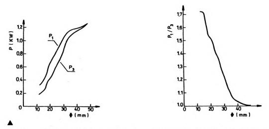
Fig 2. Laser output power vs diaphragm diameter.  $P_1$  and  $P_3$  correspond to the small signal gain (curves 1 and 3 in Fig. 1, respectively)
