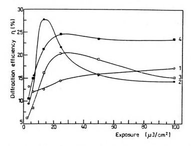
Fig. 2. Variations of the diffraction efficiency with exposure for photographic phase gratings produced with ICP 163 developer and the bleaches 1, 2, 3 and 4
