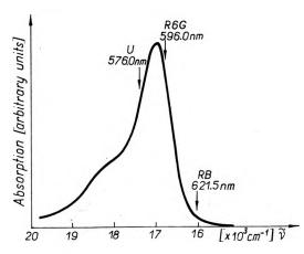
Fig. 5. Absorption spectrum of the ethanolic DODCI solution. Arrows indicate the maxima of free running uranin, rhodamine 6G and rhodamine B lasers
