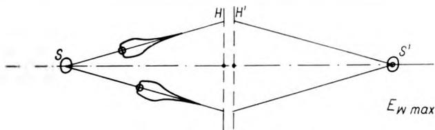
Fig. 6.  $N$  bubbles occurring in an optical system; their maxima of background illumination intensities are summed up in the image plane
