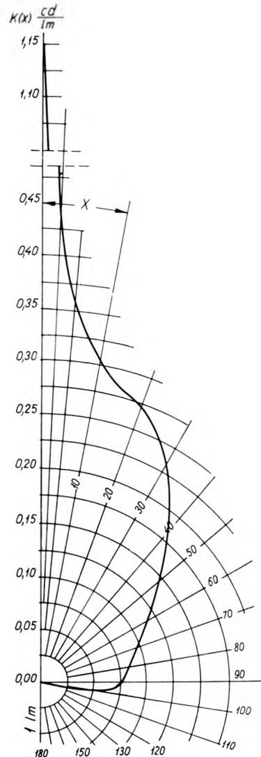
Fig. 2. Experimentally determined indicatrix of directional luminous intensity of a bubble in a borosilicate glass piece
