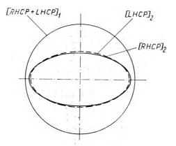
Fig. 12. Experimental checking of the dividing system of the detection unit for the detectors  $1\theta$  and 11.  $[RHCP + LHCP]_1$  – entering right left circularly polarized light,  $[RHPC]_2$ ,  $[LHCP]_2$  – outgoing right and left elliptically polarized light
