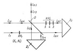
Fig. 4. First design of the interferometer presented schematically
