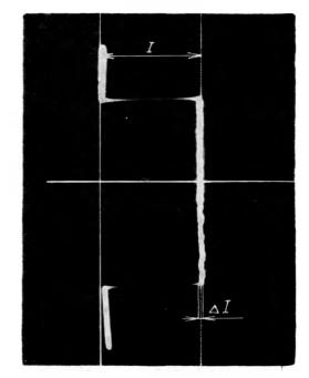
Fig. 3. Interference of two circularly polarized beams of the opposite handedness and the same intensity, without the analyser before the detector entry
