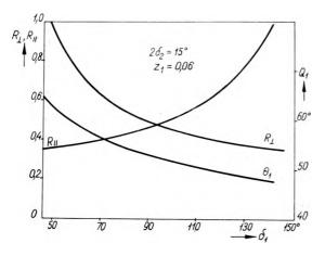
Fig. 5. Graph determining the values  $\delta_1$  and  $\theta_1$ of the first phase retardation plate  $RP_1$  depending on the dividing layers properties  $2 \delta_2$ ,  $R_{\parallel}$ ,  $R_{\perp}$ ,  $Z_1$
