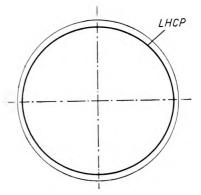
Fig. 8. Form of the nearly circularly polarized light of the measuring of the beam [LMCP] outgoing from the experimental interferometer
