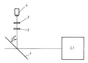
Fig. 13. Layout of the arrangement for elimination of the reference beam as a part of the system for signalization of the beam interruption
