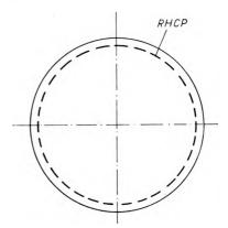
Fig. 7. Form of the nearly circularly polarized light of the reference beam [RHCP] outgoing from the experimental interferometer
