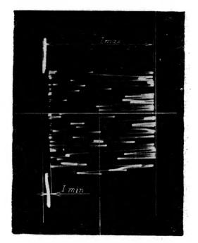
Fig. 2. Interference of two circularly polarized beams of the same handedness and intensity, without the analyser before the detector entry
