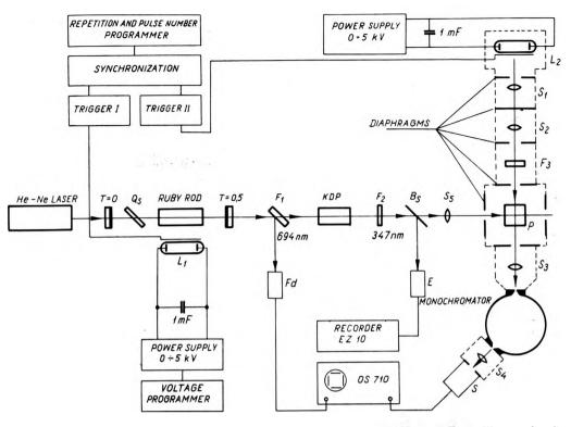
Fig. 1. Optico-electronic scheme of the measuring system:  $F_1$ ,  $F_2$ ,  $F_3$  – filters,  $S_1$ ,  $S_2$ ,  $S_4$  – spherical quartz lenses,  $S_3$ ,  $S_5$  – cylindrical quartz lenses,  $Q_8$  – passive Q-switch, Bs – beam splitter,  $L_1$  – G-422 flash lamp pumping ruby rod,  $L_2$  – analyzing light source, P – sample, E – photoelectric energy meter, S – photoelectric probe with photomultiplier, Ed – photoelectric probe with FDWCZ photodiode
