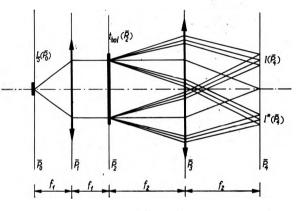
Fig. 1. Scheme of partially coherent reconstruction of Fourier holograms
