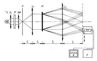
Fig. 3. Diagram of an arrangament for partially coherent reconstruction of Fourier holograms, and measurement of the intensity distribution in the image:
