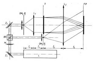
Fig. 2. Diagram of an arrangement for registration of Fourier holograms:
