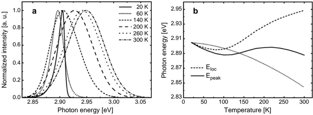
Fig. 3. The simulated luminescence spectra  $I(E)$  (a), and emission energies  $E_{loc}(T)$  and  $E_{peak}(T)$  under various temperatures for InGaN MQW sample; the dotted line represents the results calculated by the Varshni law (b).
