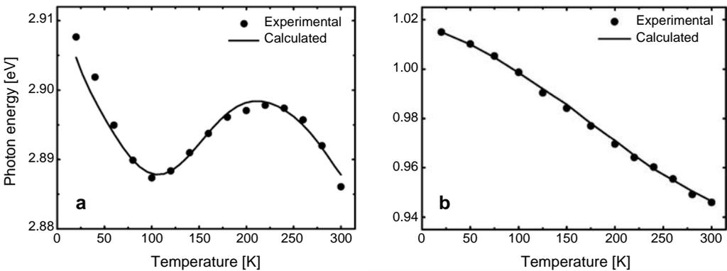
Fig. 1. Temperature dependence of peak position of PL spectra from InGaN/GaN MQW sample (a), and InAs QD sample (b). The solid lines are fitting curves based on the rate-equation model with fitting parameters listed in the Table.
