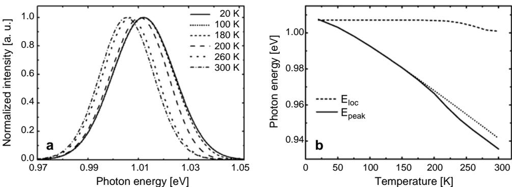
Fig. 4. The simulated luminescence spectra  $I(E)$  (a), and emission energies  $E_{loc}(T)$  and  $E_{peak}(T)$  under various temperatures for InAs QD sample; the dotted line represents the results calculated by the Varshni law (b).
