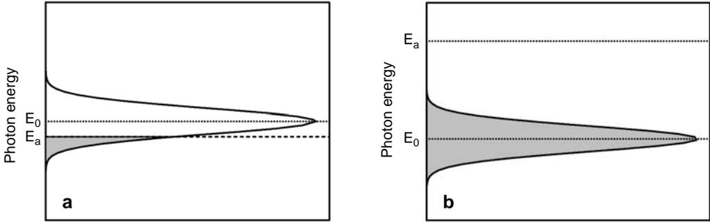
Fig. 2. Schematic diagrams of electronic structures for InGaN MQW sample (a), and InAs QD sample (b).
